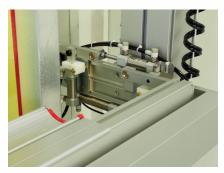
Pneumatically Controlled Coating Carriage
