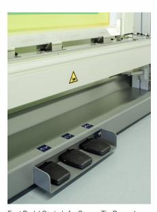
Foot Pedal Controls for Screen Tie-Bar and Stretchers
