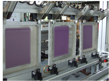
Fasteners for Multiple Simultaneous Screen Treatment (Option Z)
