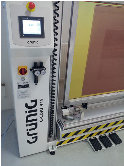
Raised Floor Base for Easier Screen Handling (Version A20)
