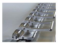
Clamps Positioned on Guideway
