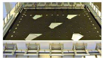
Supporting table with perforated grid and freely positioned angular stop pieces
