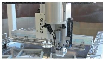
Multi-functional gluing head: measuring, gluing and curing
