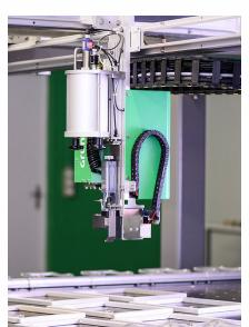
Automated Gluing and Curing Head
