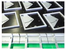
Angle Blocks for Easy Screen Alignment (Option W)
