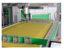
Complete G-STRETCH 275 UV Bond LED Stretching and Gluing System
