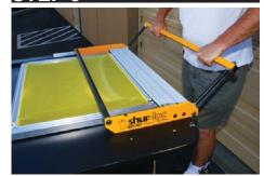
The stretcher is now completely assembled and ready to use with the shur-loc® "E-Z" Frame.
