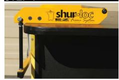
Position the stretcher on the edge of the table top or board allowing the handle to rotate 180°.
