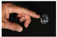
Install the washers and wing nuts under the table top or board and tighten.
