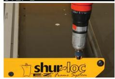
Use the drill motor with the 1/4" bit to drill through the table or board using the bolt holes as a vertical drill jig.
