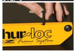
Install the 4" 1/4-20 bolts through the holes that were drilled in the table top or board.
