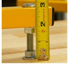
Set the height of the Safety Bar to 1 3/4" from the table top using the secondary nut and washer. Once you have set this close, it will not need to be adjusted. Make sure that the bolt passes through the table.
