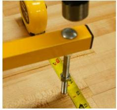
Position the bar about 13 1/2" from the edge of the table that you wish to stretch from. Strike the bolt with the hammer to "mark" the positioning. Be sure to strike both sides of the safety bar.
