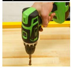
Using the 7/16" drill bit and motor, drill out both 'bolt marks' that you made using the Safety Bar and hammer. Drill completely through the table or board you are using as you will need to fasten a wing nut to the bolt.
