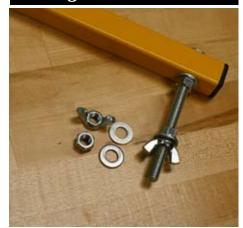
You will need a hammer, drill motor, 7/16" drill bit, and tape measure to complete this installation. Please remove the tension tool from the package and locate the Safety Bar. Remove the wing nuts from both bolts.
