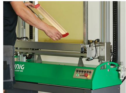
Installation of coating trough
