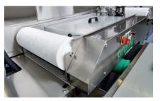
Closed-Circuit Tank with Inclined Filter
