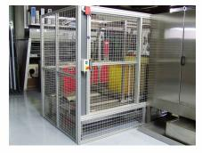
Loading/Unloading Magazine with Protective Cage
